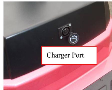
Recharge battery only when the key is in off position. When indicator is in low status, this confirms the battery needs recharging.
